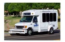
every public street under the Village's jurisdiction. IMS will perform a surface condition survey using a road surface tester mounted on a specialty vheicle that will collect information on pavement roughness, cracking, texture and distress to provide continouse and accurate condition of the Village's street network. The final report delivered to the staff will be used to help prioritize maintenance street resurfacing in the coming years.
